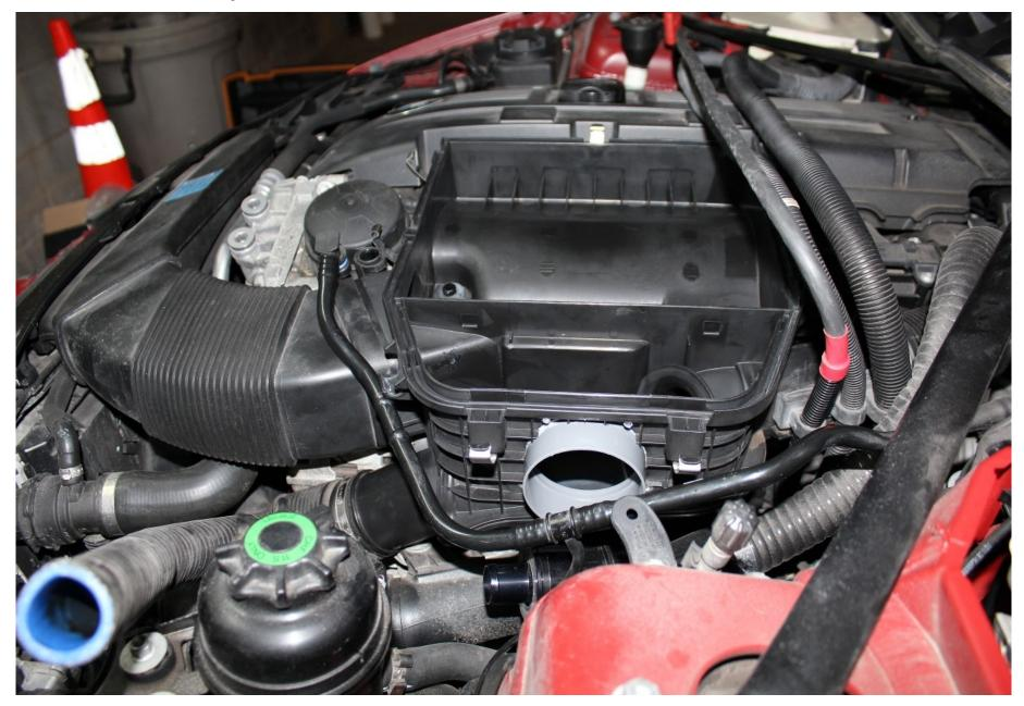
Using a hair drier, heat up the plastic connector on the brake booster hose. Then, very carefully, turn twist the hose in such a way so that the nipple points horizontally and not downwards anymore. This will give you additional clearance for the Spectre 3-inch pipe. Warning: Be careful not to break off the nipple!
