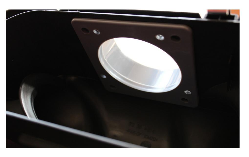
Test fit the rivets and make sure everything fits correctly! Note: I installed two of the rivets from the inside of the airbox and two from the outside:
