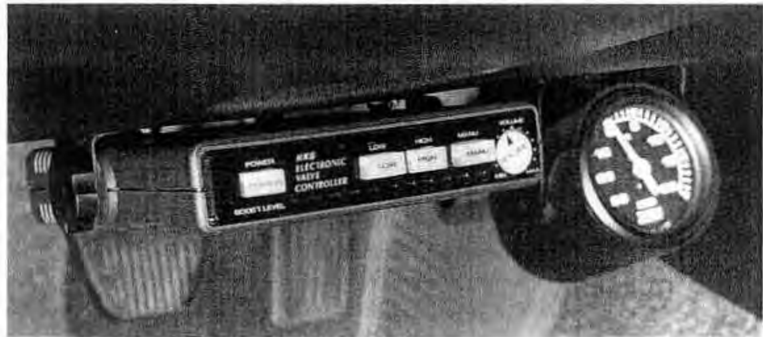
Fig. 12-20. The HKS Electronic Valve Controller is a multi-level boost-change device that also produces faster boost rise by blocking the signal to the wastegate until near-maximum boost is achieved.
