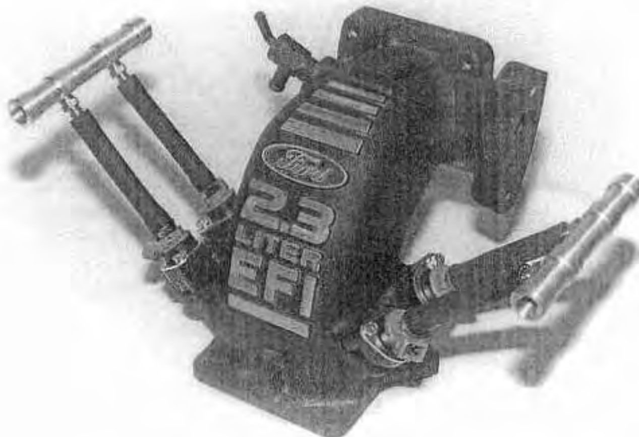
Fig. 7-13. Four staged secondaries can be programmed to operate when under boost.
