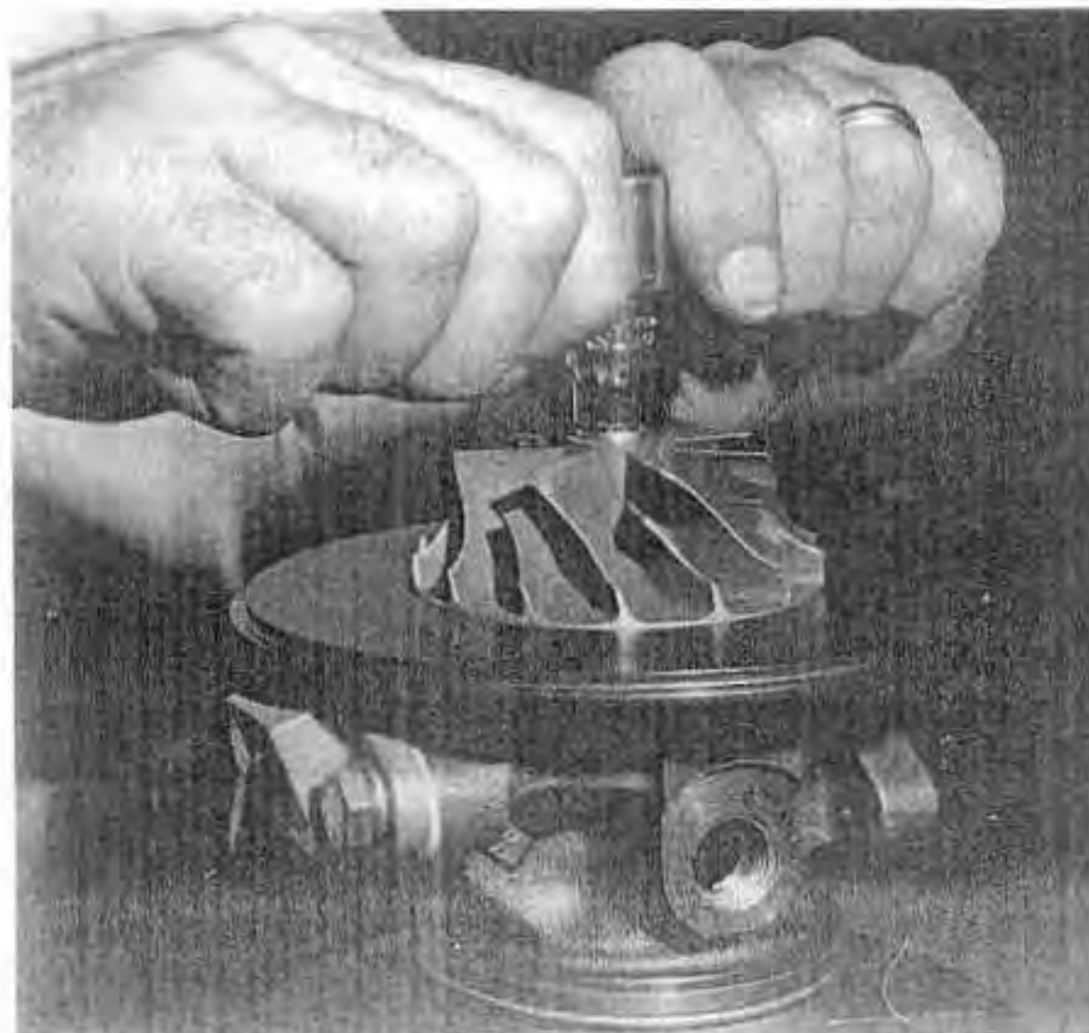
Fig. 15-4. One way to tighten the compressor retaining nut. Using a T handle will eliminate bending loads in the turbine shaft.
