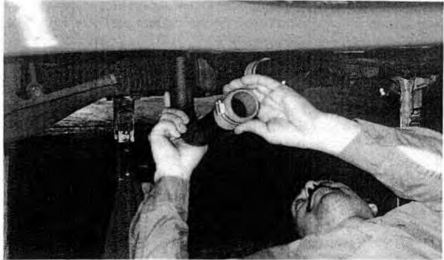
Fig. 18-17. With the turbo and intercooler in position, the interconnecting tubes can be installed.
