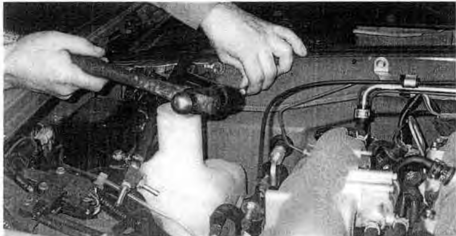
Fig. 18-22. The rising-rate fuel pressure regulator conveniently mounts to the firewall. Drilling the mount holes accurately requires a drill dimple.
